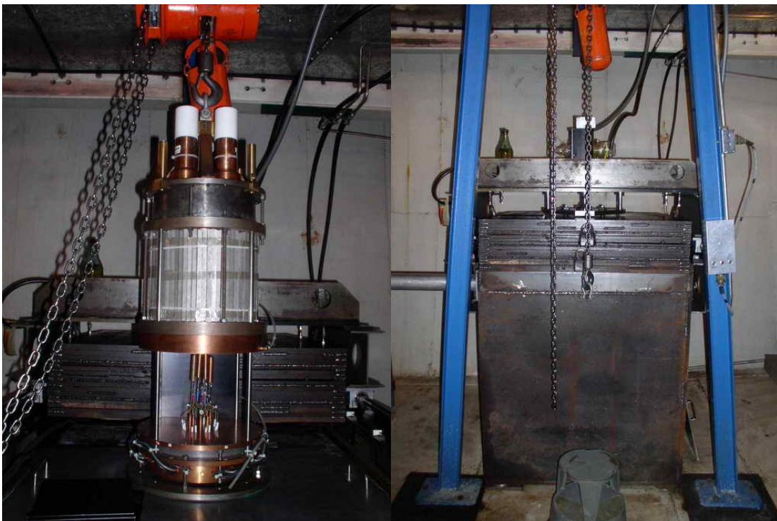
Fig. 3. The counters in the well of the NaI detector (on the left), the large passive shield (on the right).
