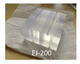
5 × 5 × 5 cm<sup>3</sup> PVT cubes – Non-flammable scintillator Cubes are optically separated using Tyvek wraps <sup>6</sup>LiF:ZnS(Ag) screens for neutron identification Light collected through optical fibers and silicon photomultipliers (SiPMs require low-voltage)
