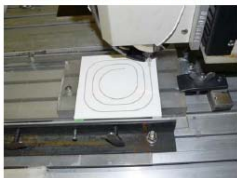
Groove for WLS fiber
